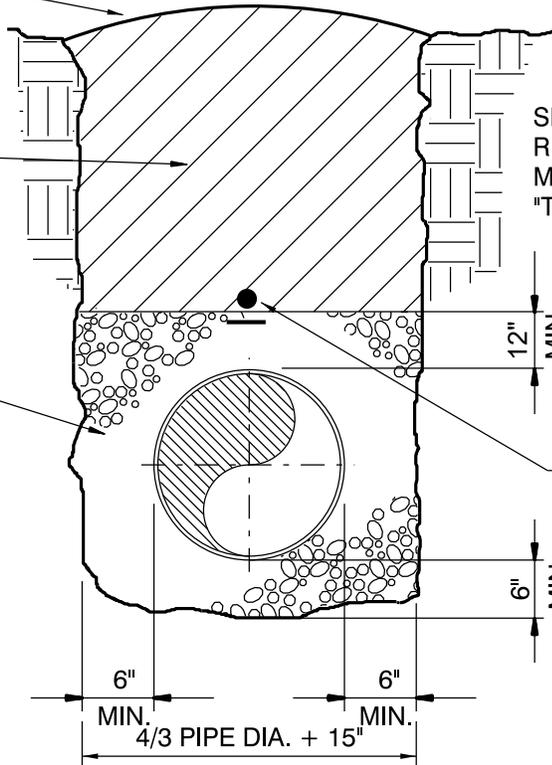
DETECTION TAPE & PVC COATED 12 GAUGE TRACER REQUIRED FOR PVC PIPE. TRACER SHALL BE STUBBED INTO ADJOINING VALVE BOXES.
