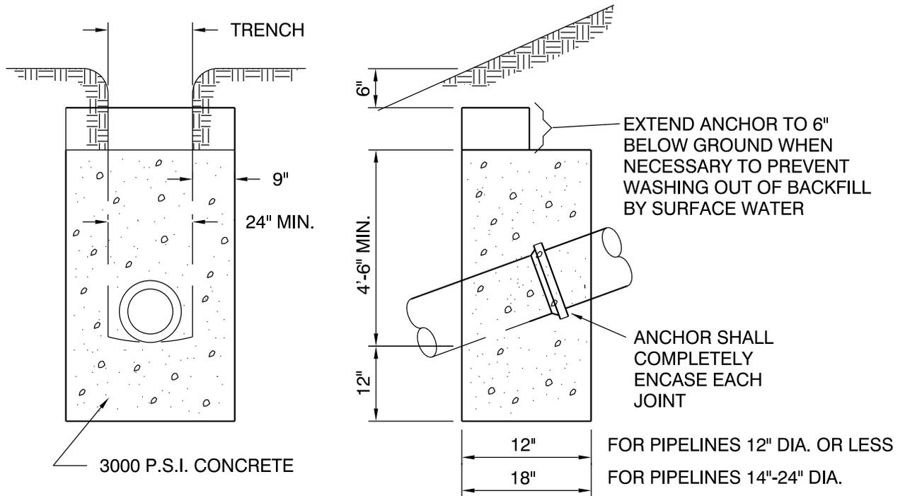
NOTE: PROVIDE NO ANCHOR ON GRADES LESS THAN 20% UNLESS NOTED.
