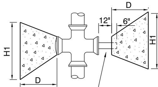
PLUG PIECE OF 6" PIPE TO BE USED ONLY WHEN SPECIFIED ON LAYOUT SHEET
